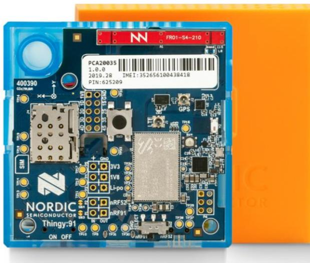
**Figure 1** – TRIO mXTEND™ chip antenna component, member of the Virtual Antenna™ family, (component in red) embedded in Thingy:91 by Nordic Semiconductor which is a multi-sensor prototyping kit ideal for kick starting cellular IoT projects
